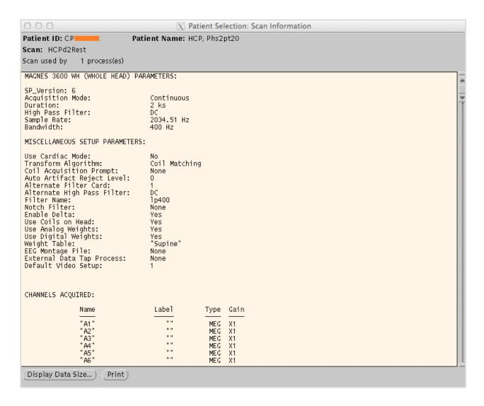
In the Data File Information screenshot, Channel reference information is given for the first few channels. A complete listing of this info is contained in the headers, which are accessible by reading the data into MATLAB. Because we record continuous data, "epoch information" will reflect the whole scan as a single epoch. Points (times) sample period = epoch duration.
